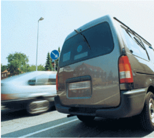
Figure 3: Mobile speed enforcement technology. The camera is placed in the back of the van. The picture is taken of the front of the oncoming car.
